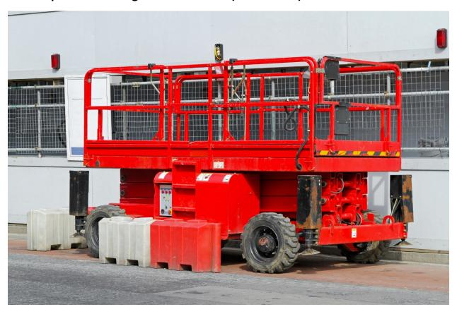
All Scissor lifts will be equipped with standard guardrails. In addition to the guardrail provided by the manufacturer, the scissor lift must be equipped with anchorages meeting the ANSI Z359 Fall Protection Code.
